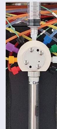
Dispensing syringe with 9-port valve and mixing chamber - dispensing syringes from 250 µl to 20 mL
