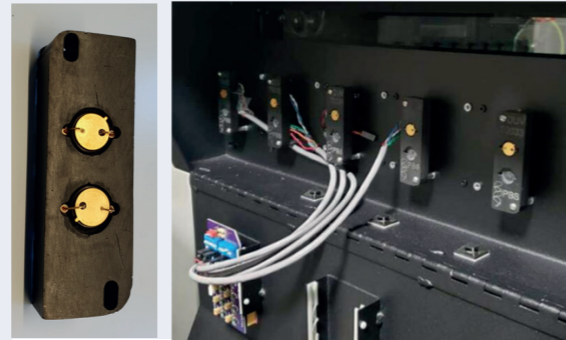
Single or dual-wavelength detection based on LED-technology with 280 and / or 254 nm
