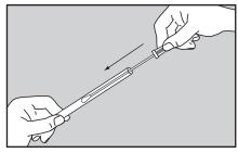
After sampling is complete, securely insert the swab back into the swab tube and transport to the lab for inoculation. Plate the letheen broth swab solution as soon as possible. Go to step 7 of the Inoculation Methods Section.
