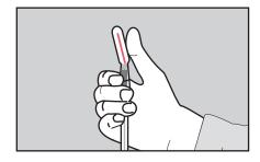
At the sampling location, prepare the swab by holding it with the bulb end near your thumb. Bend the red snap valve at a 45° angle until you hear the valve break. This allows the letheen broth to flow into the tube end and wet the swab.
