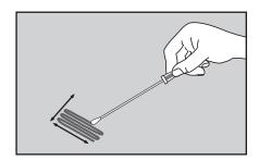
Hold the swab handle to make a 30° angle with the surface. Rub the swab slowly and thoroughly over desired surface area. Rub the swab three times over this surface, reversing direction between alternating strokes.
