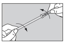
Twist and pull apart the tube end of the swab from the bulb end of the swab which contains the letheen broth.
