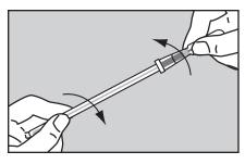
Twist and pull apart the bulb end of the swab from the tube end of the swab which contains the letheen broth.
