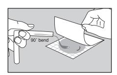
3 Use your thumb to bend the swab tube at a 90° angle at the highest mark that has diluent above it. Pour off a 1mL aliquot onto a Petrifilm plate. Repeat until the entire sample is used. Follow current industry standards for disposal.
