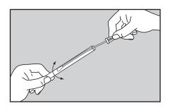
Wring out the contents of the swab tip by pressing and twisting the swab against the wall of the tube.
