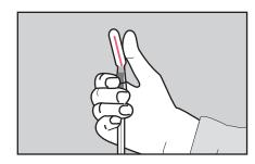
Prepare the swab by holding it with the bulb end near your thumb. Bend the red snap valve, at a 45° angle until you hear the valve break. This allows the letheen broth to flow into the tube end and wet the swab.
