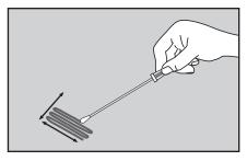
Hold the swab handle to make a 30° angle with the surface. Rub the swab slowly and thoroughly over the desired surface area. Rub the swab three times over this surface, reversing direction between alternating strokes.
