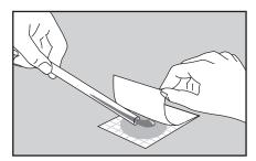
Garefully pour the entire contents of the tube onto a 3M<sup>™</sup> Petrifilm<sup>™</sup> plate. Follow current industry standards for disposal.
