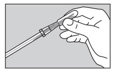
Squeeze the bulb of the swab to transfer all of the letheen broth into the tube end of the swab.
