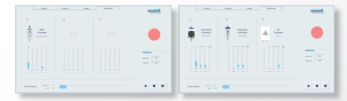
Printing menu shows real-time status of the printing machine, printed object and various other information about the object being printed. Users also has ability to pause the print anytime and change cartridge, or do anything according their protocol.
