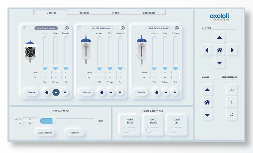
AxoSuite Control enables users to manually adjust temperature, pressure and voltage of each printhead individually, also users can do manual movement and control the cabin leds, uvs and HEPA filter that comes with the machine.
