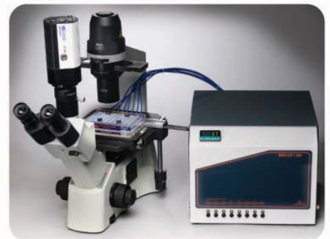
Figure 1: The BioFlux System for live cell assays under controlled shear flow.
